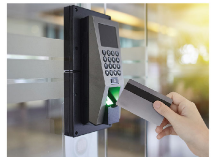
Access Control System
